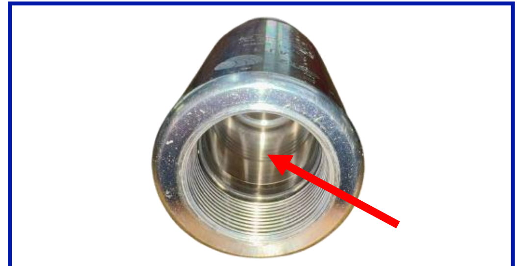
Damaged nozzle housing
