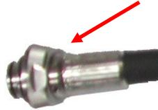
Caution: The forward jet may only be tightened using an 8 mm open-ended spanner (do not tighten hand-tight). Keep the grub screw removed in a safe place. You will need it again if you want to work without the front jet nozzle.
