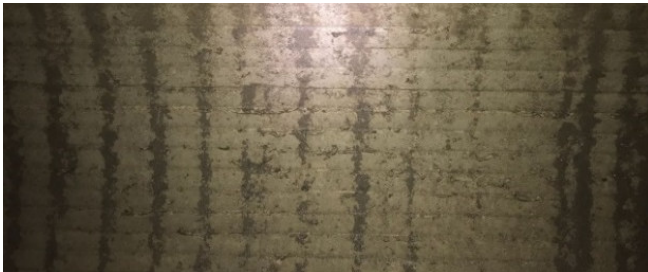
Figure 15 Streak formation in the pipe
