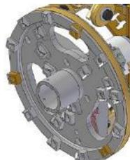
6. Coat the thread of the six Allen screws with Loctite 243 (C192). Then tighten these to a tightening torque of 50 Nm.
