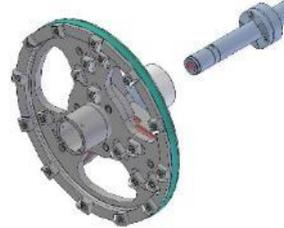
6. Undo the three screws of the cam plate
