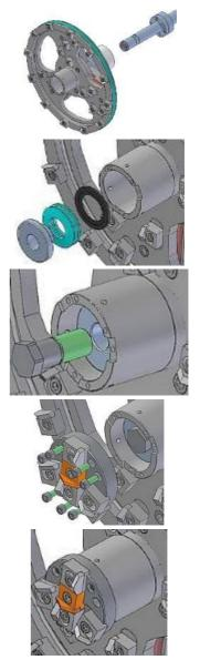
Figure 22: Change the cam plates
