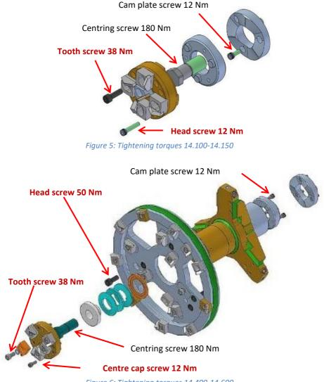
Figure 6: Tightening torques 14.400-14.600
