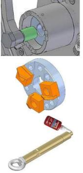
Figure 16: Mount the pull rod
