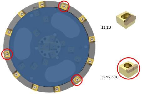
Figure 9: Cutting teeth on the outer ring
