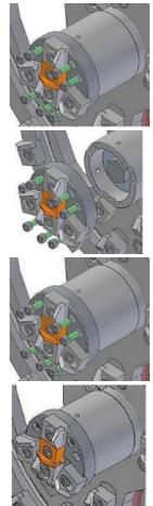
Figure 15: Disassemble and mount the centre cap
