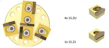
Figure 7: Cutting teeth on the centre cap
