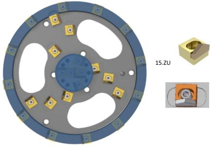
Figure 8: Cutting teeth on the inner ring
