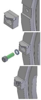
4. Tighten the screw to 38 Nm.
